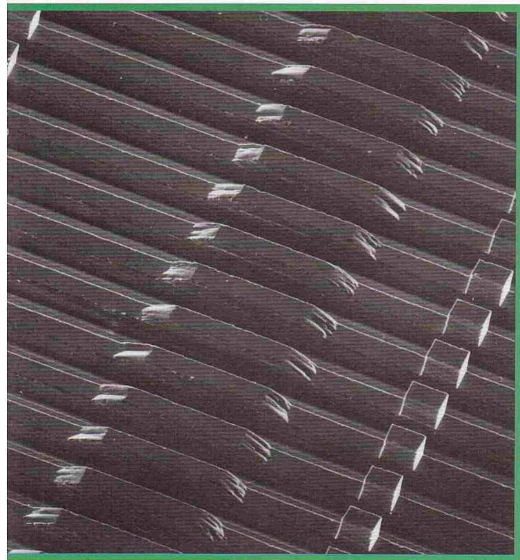
900 \mu\text{m} , fabricated in (100)-silicon with anisotropic wet etching.
