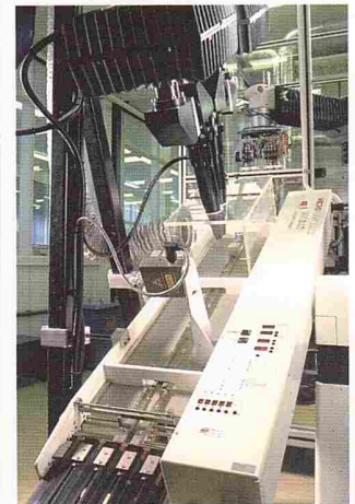
The laser printing of barcoded calibration data is one step in the automated production at Skoppum.
