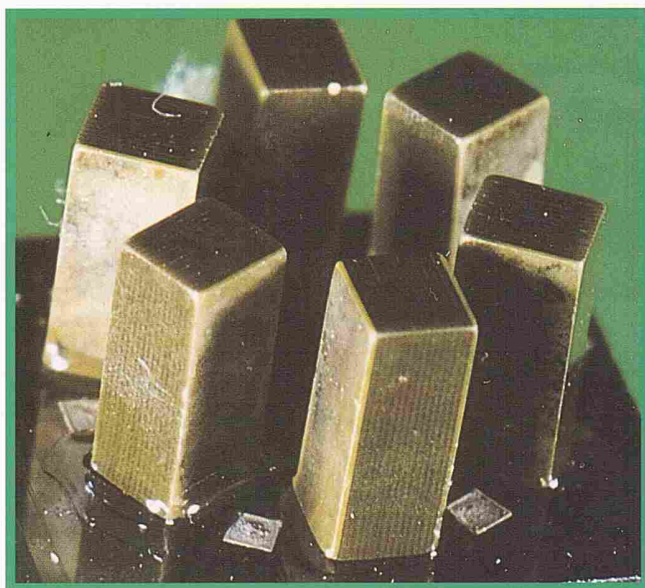
A piezoceramic stator intended for a miniature motor with diameter and height of 4 mm and 2 mm respective. (M. Bexell et al, Uppsala University, Sweden).
