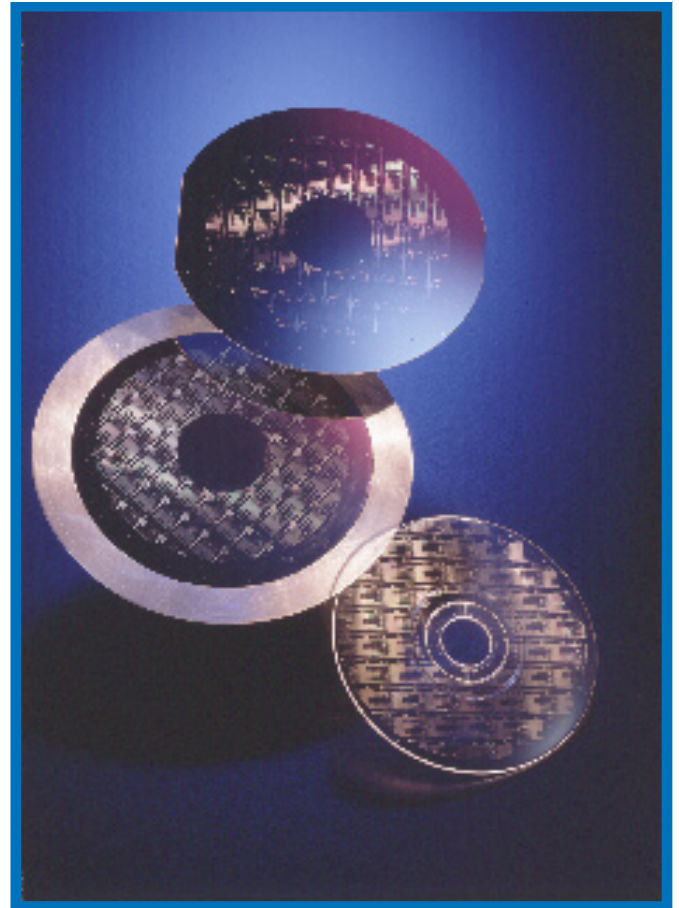
Low cost production process for fabrication of polymeric microstructures (Silicon-Nickel-Polymer). Plastic substrates with waveguide channels for fabrication of 1:4 optical power splitters were injection molded in a state-of-the-art production equipment for CDs (Cycle time about 10 seconds.) The technique is developed in co-operation between IMC and Toolux Alpha.
