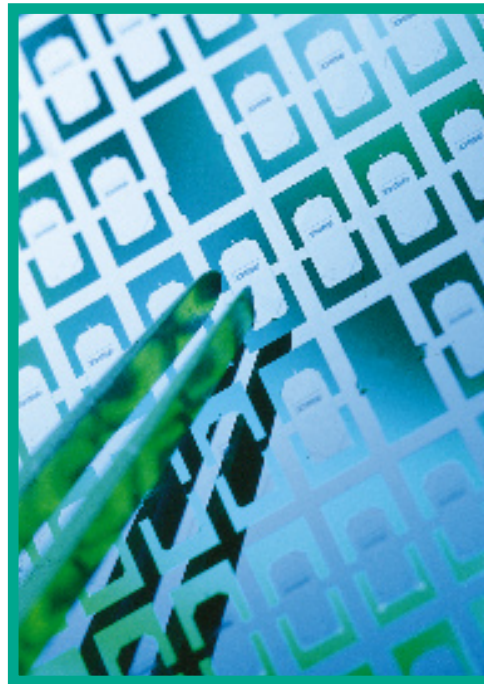
Removing commercial atomic force microscope (AFM) probes from a wafer (photo: Karsten Damstedt).
