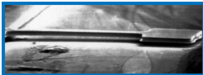
Surface micromachined InGaAs paddle on InP, made at the Laboratoire Electronique, Ecole Centrale de Lyon
