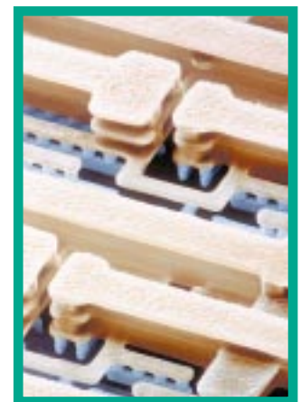
Copper leads inside a semiconductor made visible by etching away the silicon (courtesy of IBM).
