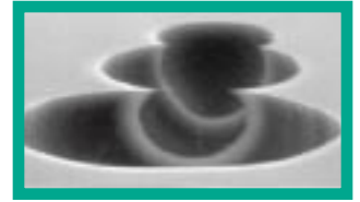
Plasma etched silicon snowman with a neck of 5 \mu\text{m} diameter.
